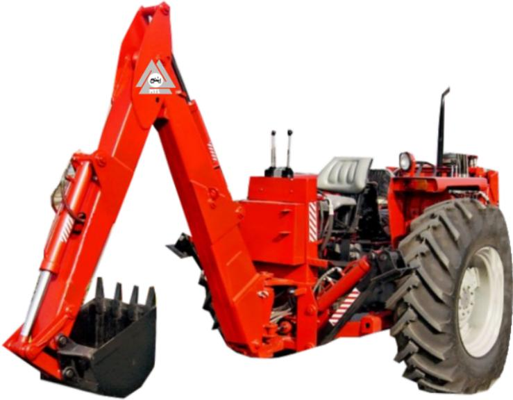
Millat Backhoe can be attached and detached from the Tractor within a little time. Can also be mounted with front attachments. Digging now made easy with speed and work efficiency.
