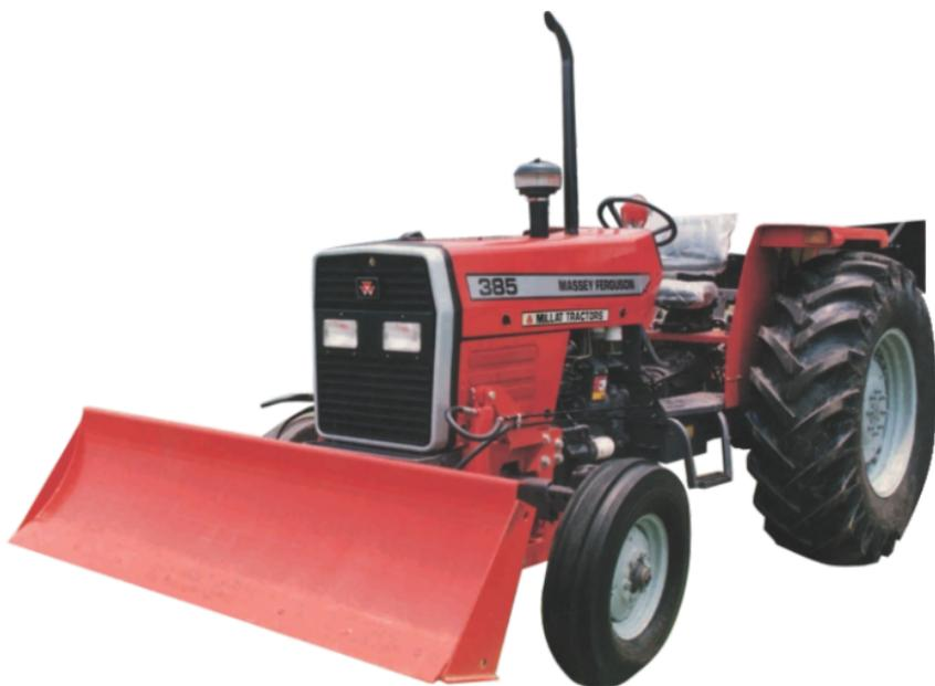
The Power Dozers are designed and built to match the performance of the Millat Tractors. They are operated hydraulically by single or twin double acting rams. The points of attachment of the dozer to the tractor are reduced to an absolute minimum and the mounting brackets, once fitted, can be left in position enabling the sub-frame and blade to be quickly removed and attached. The blade is fitted with a reversible and replaceable cutting edge of high carbon steel.
