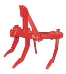
The Chisel Plough is primary tillage deep plough, working upto 20" to ensure development of crop root system at proper depth and environment. It is an ideal implement where top soil is fertile but subsoil is not productive. The Chisel Plough increases natural fertility of soil as deep tillage provides enough circulation of air, moisture, and sunlight into soil.
